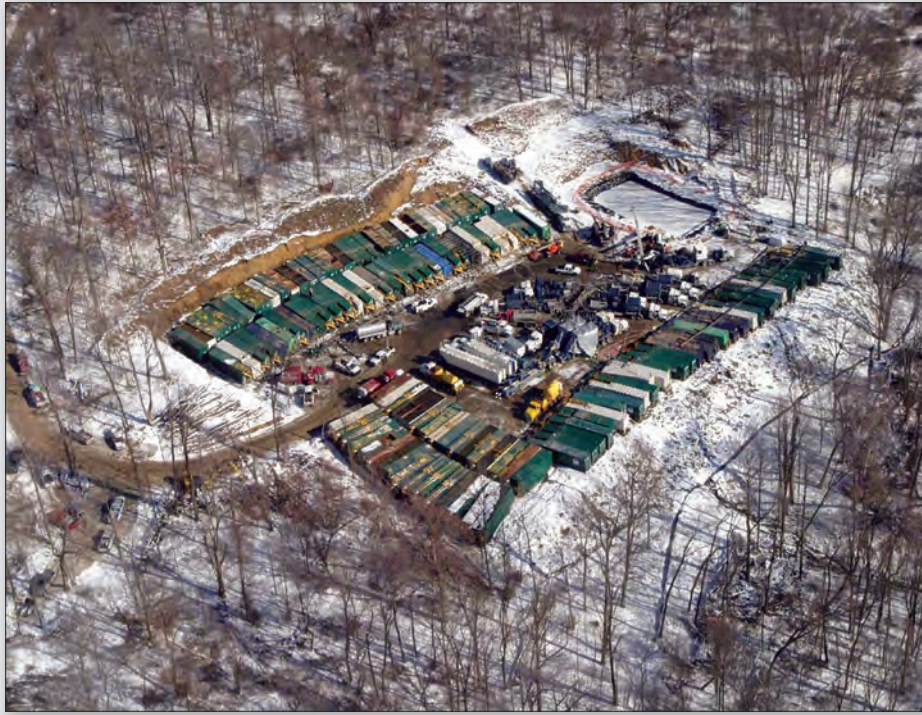
Figure 6. A hydraulic fracturing stimulation in 2007 on a Marcellus Shale gas well showing the amount of equipment involved.
